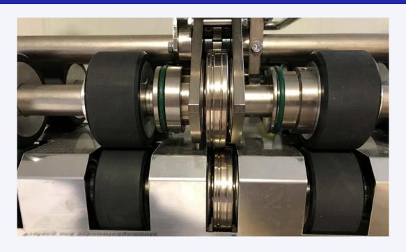
2 Scoring mechanism: They all are equipped with male and female scoring tools and can be used interchangeably
